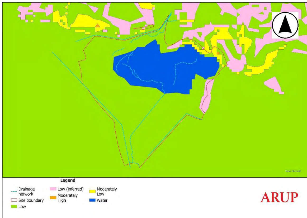
Figure 7-1: Geological Survey of Ireland Landslide Susceptibility mapping for Fin Lough (Offaly)
